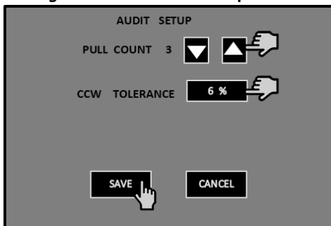
Figure 33: DTT Audit Setup Screen B
