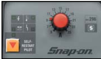
Faceplate showing Depth-of-Cut adjustment dial
