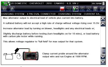
Fast-Track® Guided Component Tests in the tool, include guided test procedures, automatic meter set-up, connection tips, connector diagrams, waveform library, test values
