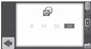
Figure 17: Auto Shut Down Display
