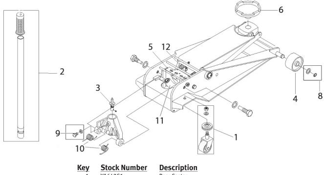
Rear Caster Handle, Complete Universal Joint Front Wheel Power Unit Saddle Washer/Retaining Ring Handle Bolt kit Handle Return Springs (Left & Right) Pump Piston Assembly 2 each Return Springs
